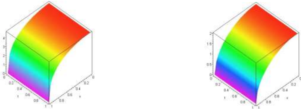
Fig.1. The profile of the distribution of the normalized flux density b(x, t) at different times t=0.1, 0.2 for n=1 .
